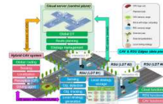
Fig. 1. LDT-based hybrid autonomous driving system architecture.
